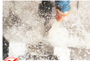
Machining with flood coolant
